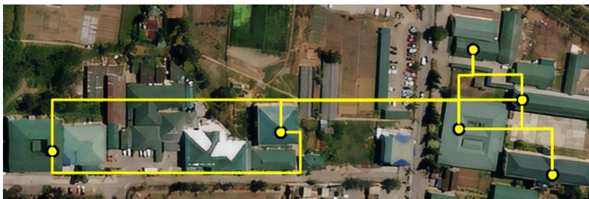
Figure 6. Proposed Fiber-optic Network Physical Layout South Main Campus.
