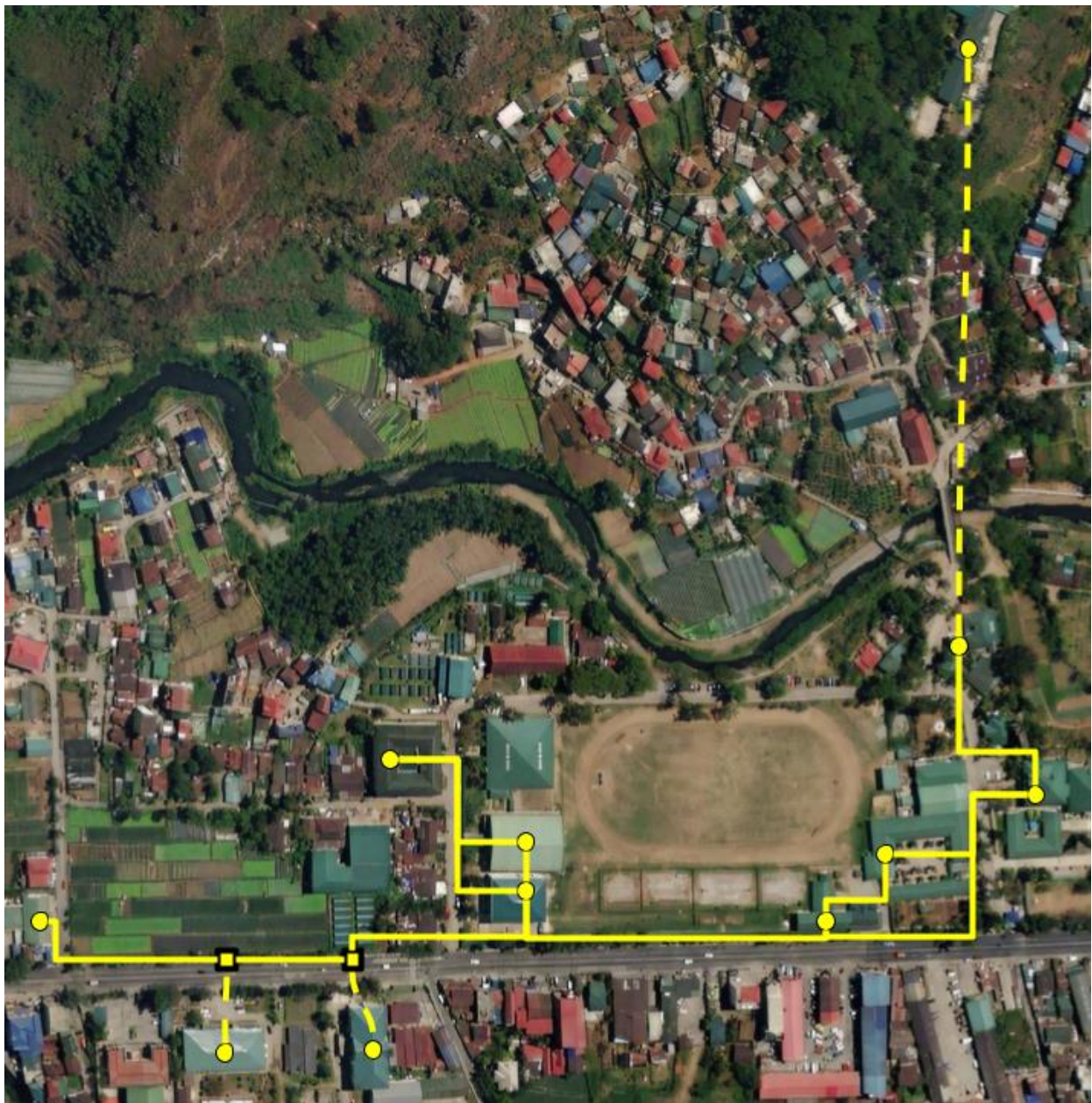
Figure 4. Proposed Fiber-optic Network Physical Layout North Main Campus.
